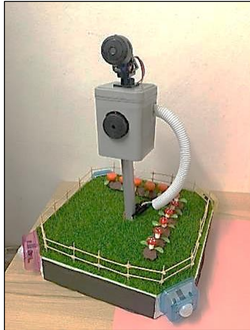
Figure 7: Final prototype of Animal Intrusion Detection and Monitoring System using IoT
