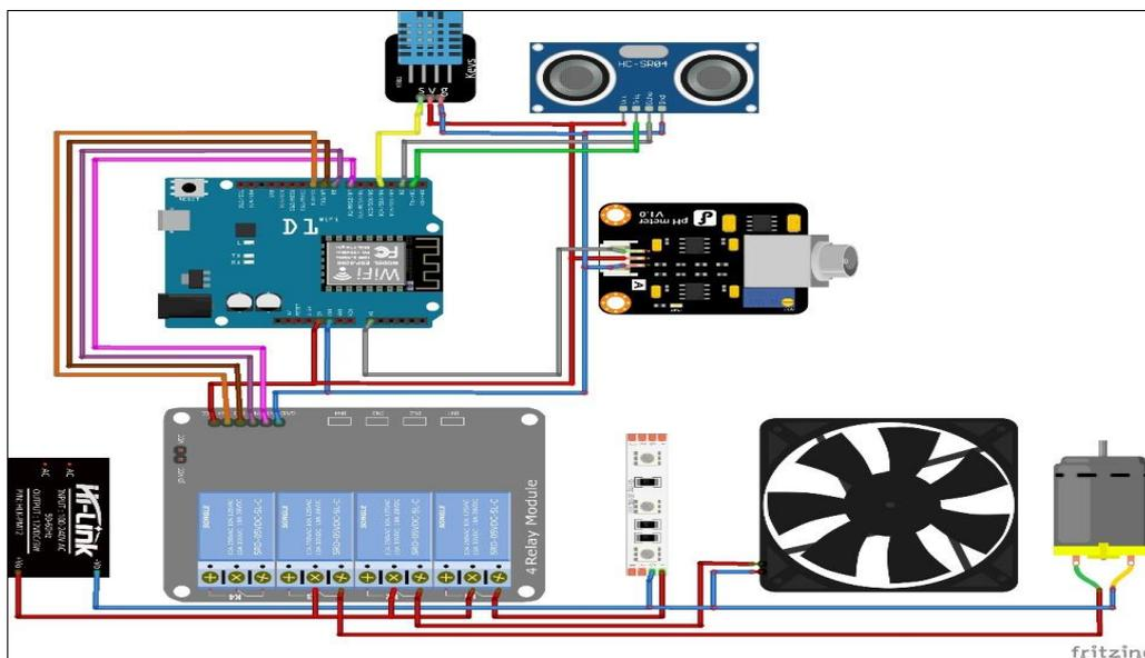
**Figure 2: The circuit diagram of vertical hydroponic farming system**
