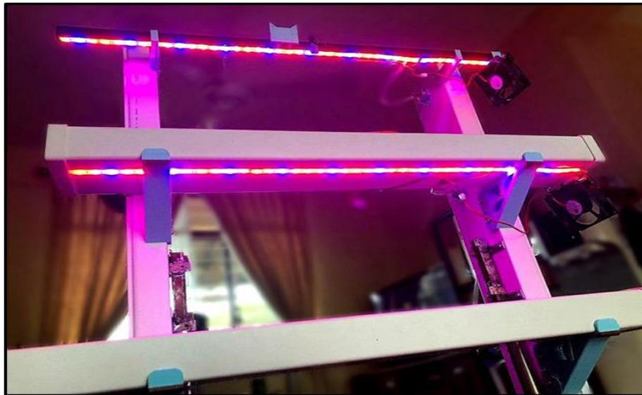
**Figure 7: The grow light and ultrasonic sensor placement in prototype**
