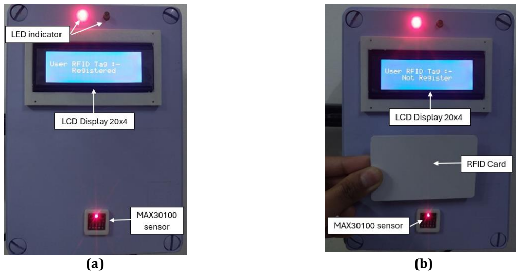
Fig. 7 LCD Display for user status (a) Registered user (b) Unregistered User
