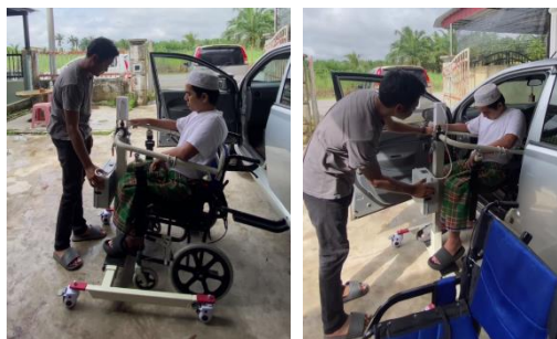
Fig. 17: Patient being transferred from wheelchair to car seat and vice versa
