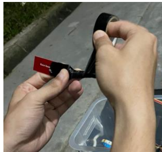
Fig. 4 Water level sensor sealing process
