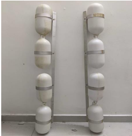
Figure 8. G-412 buoy with aluminum rod
