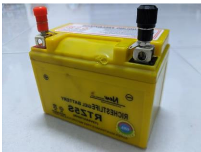
Figure 3. 12V lead-acid battery
