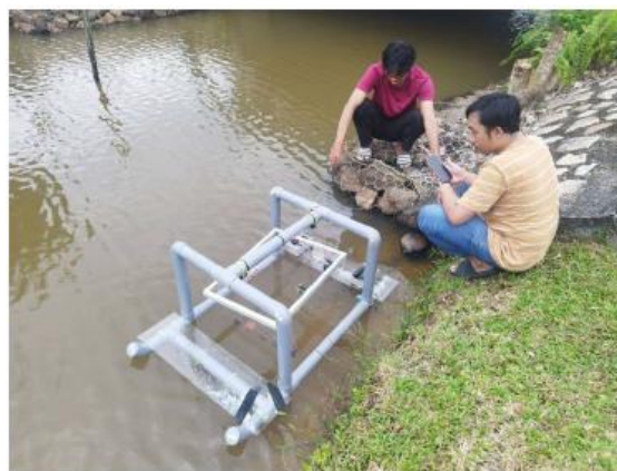
Fig. 5 Data capturing vehicle platform with research equipment floating on the water surface
