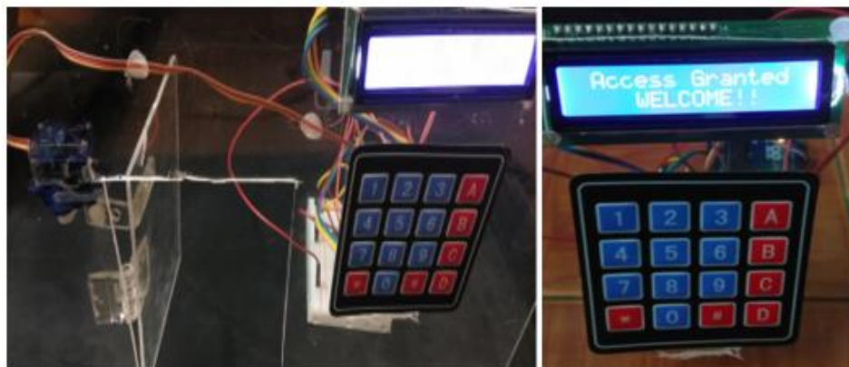
Figure 6: Access granted if password is matched and the door will unlock automatically
