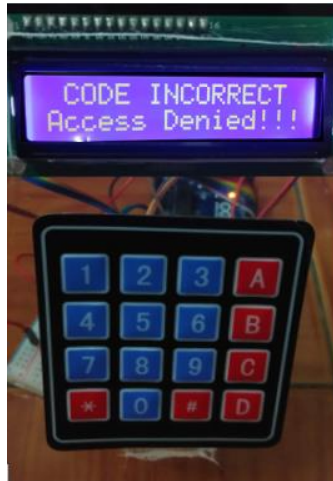
Figure 7: Displayed message when guest key in incorrect password and thus denied access by the system
