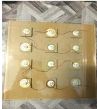
Fig. 5 Series connection of 12 piezoelectric discs
