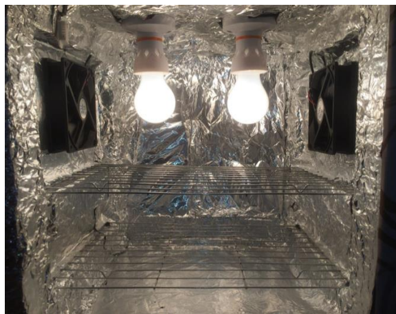
Figure 4: After sealed with aluminum foil and added fans and bulbs
