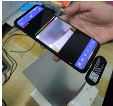
Fig. 4 Reading temperature using thermal camera onto aluminum plate
