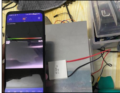
Fig. 6 Conducting evaluate experiment on the Peltier module
