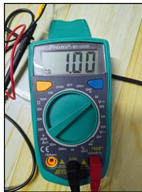
Fig. 7 Voltage reading on a unit Peltier
