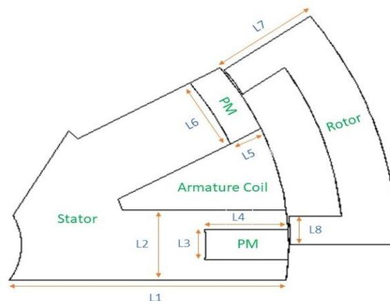
**Figure 4 : Defined parameter L1 to L8 for design modification.**
