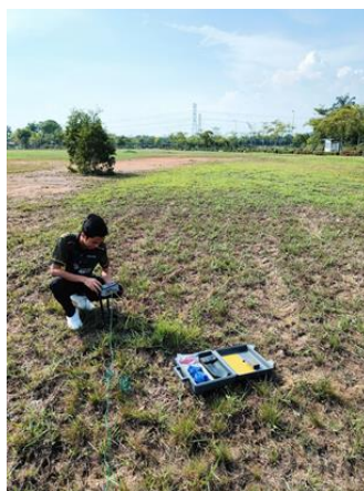
Fig 3 Taking measurement for the grounding resistance
