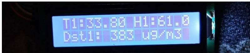
Fig. 6(d) Data for temperature, humidity, and particulate matter displayed at TF College
