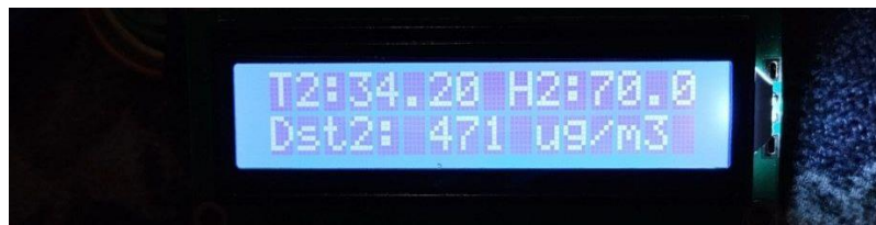
Fig. 6(e) Data for temperature, humidity, and particulate matter displayed at PTTA
