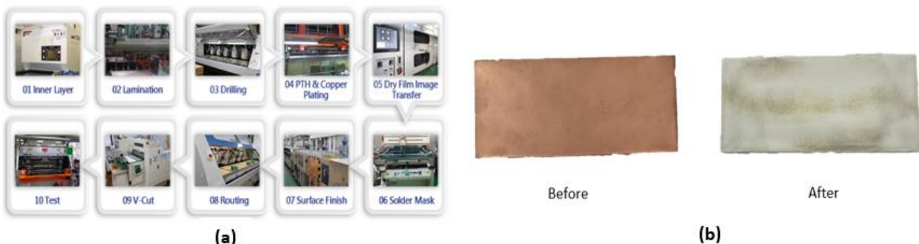
Fig. 4 Fabrication and etching (a) Fabrication flow; (b) Etching process
