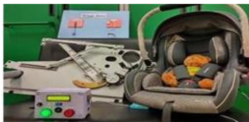
Fig. 2 Prototype car seat alert system using IoT [6]
