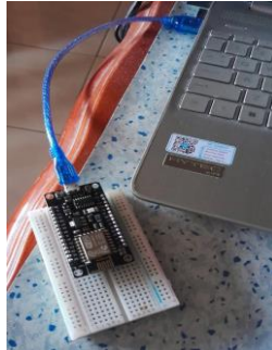
Fig. 7 Wi-Fi connected to NodeMCU ESP32
