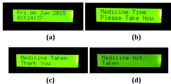
Fig. 10 Display on the LCD (a) When time interval to take medicine; (b) When the time interval to the medicine time; (c) When the time interval to the medicine taken; (d) When the time interval for the medicine is not taken
