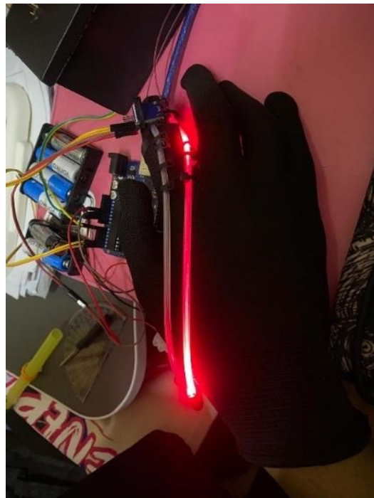
Fig. 6 Hand position to take reading optical fibre at side placement
