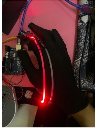
Fig. 3 Hand position to take reading optical fibre at top placement
