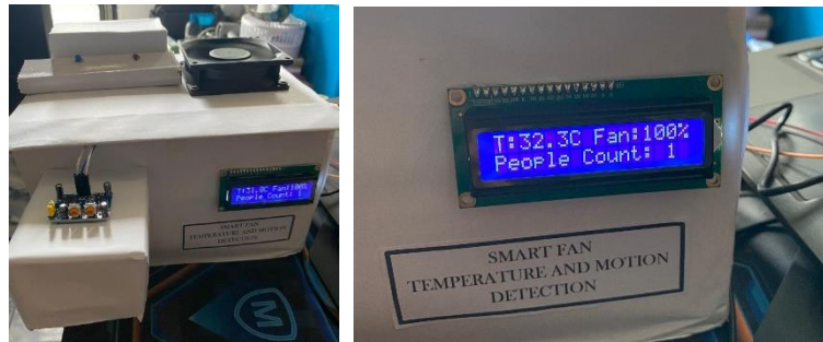
Fig. 5 Count > 0 , fan switch turns on, count = 1
