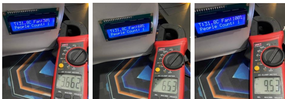
Fig. 6 Measure voltage fan speed using multimeter
