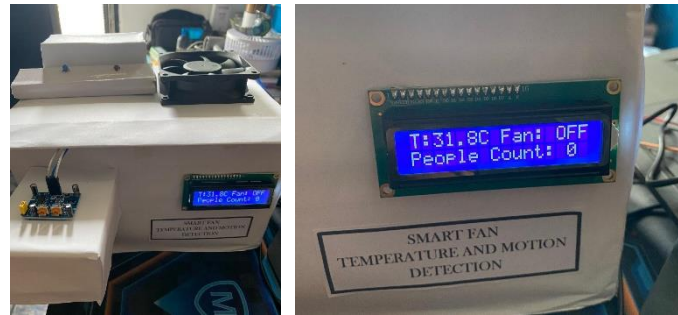
Fig. 4 Count = 0 , fan switch turns off
