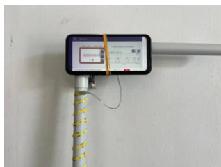
Fig. 12 Mobile Phone Placement on Cane Handle for Vibration Measurement
