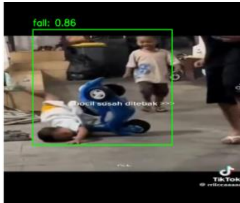
Fig. 15 Detection output of a child fall in a multi-subject scene using an adult-trained YOLOv9 model
