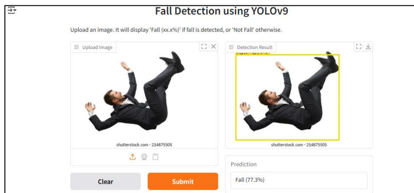
Fig. 11 GUI output of adult fall detection. The fall is successfully identified and labeled with a confidence score
