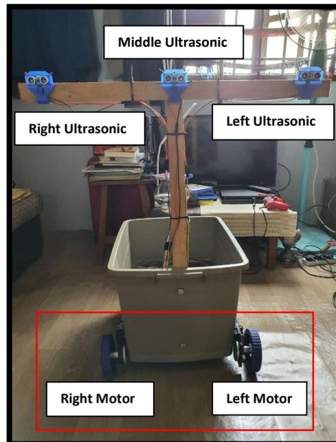
**Figure 5: Positioning of Ultrasonic Sensor and Power window motor**
