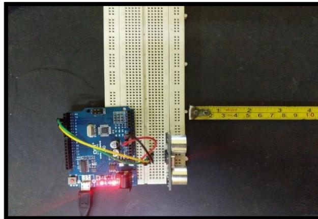
**Figure 3: The Ultrasonic Sensor Measurement and Accuracy Test**
