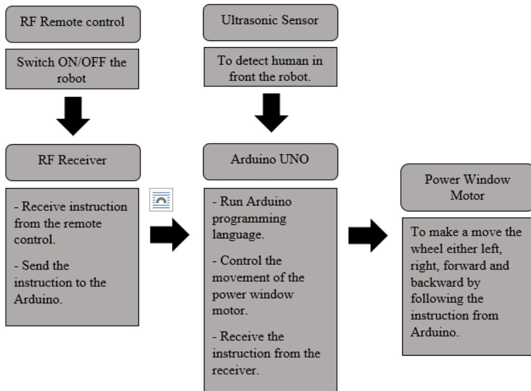
Figure 2: The block diagram for smart bag carrier by using Arduino
