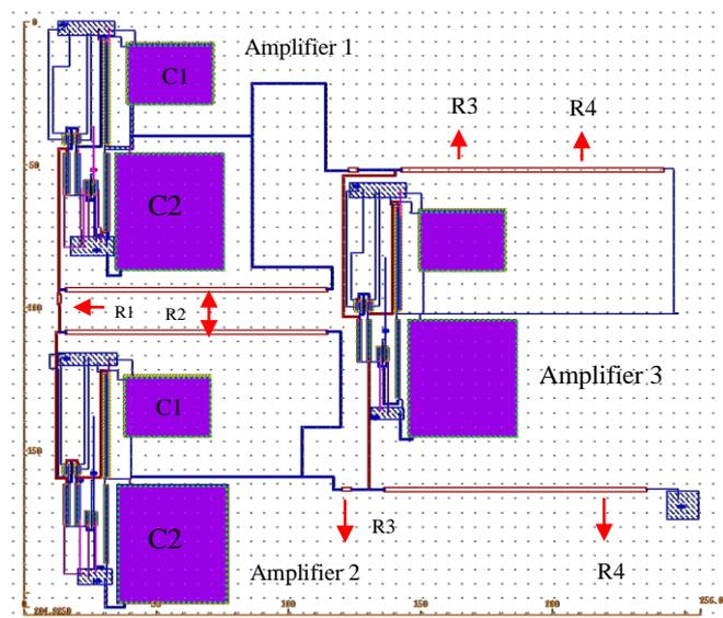
**Figure 9: Layout of proposed amplifier**
