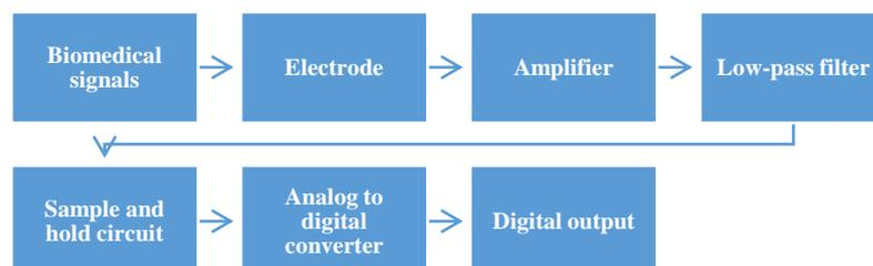
**Figure 2: Biomedical electronics detecting system blocks**
