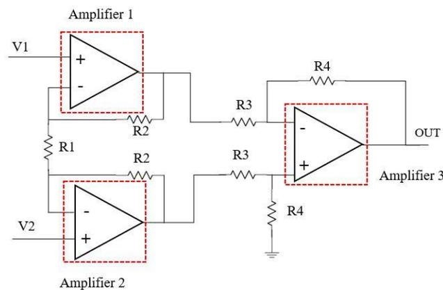
**Figure 1: Schematic diagram of instrumentation amplifier**
