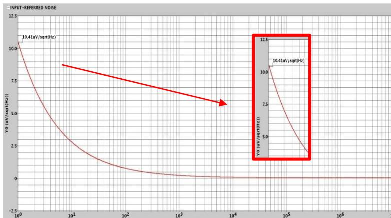
**Figure 7: Input referred noise of instrumentation amplifier (Pre-layout)**
