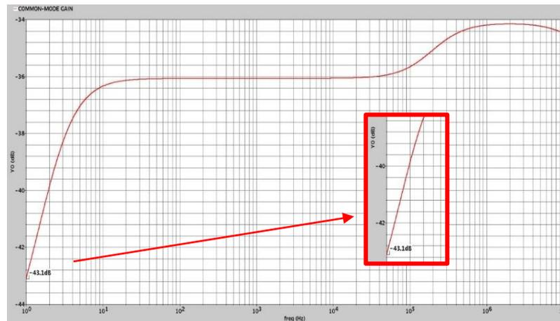
**Figure 8: Common mode gain of the instrumentation amplifier (Pre-layout)**
