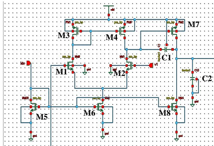
Figure 3: Schematic of two-stage CMOS op-amp
