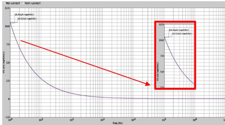
Figure 11: Input referred noise of instrumentation amplifier. (Pre-layout & Post-layout)
