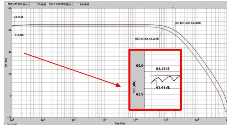
Figure 10: Differential gain of the instrumentation amplifier (Pre-layout & Post-layout)
