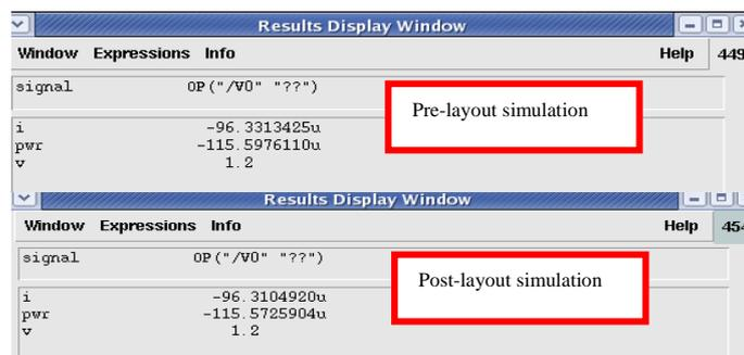
**Figure 13: Power dissipation of instrumentation amplifier (Pre-layout & Post-layout)**
