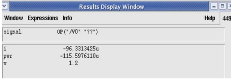
**Figure 6: Power dissipation of instrumentation amplifier (Pre-layout)**
