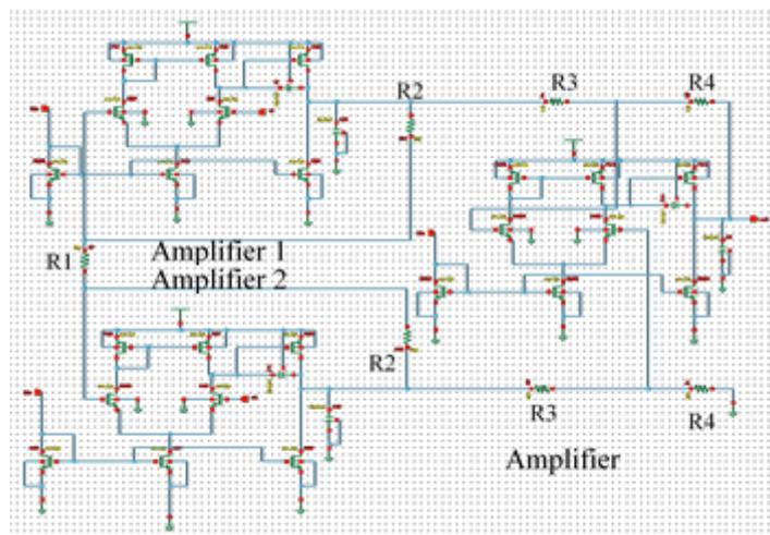
Figure 4: Schematic diagram of proposed amplifier
