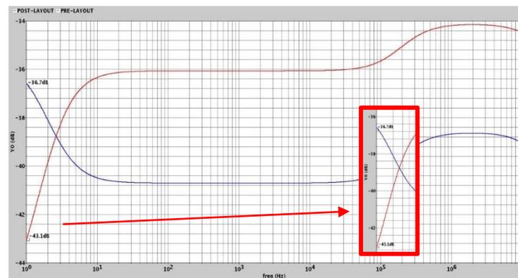
Figure 12: Common mode gain of the instrumentation amplifier (Pre-layout & Post-layout)
