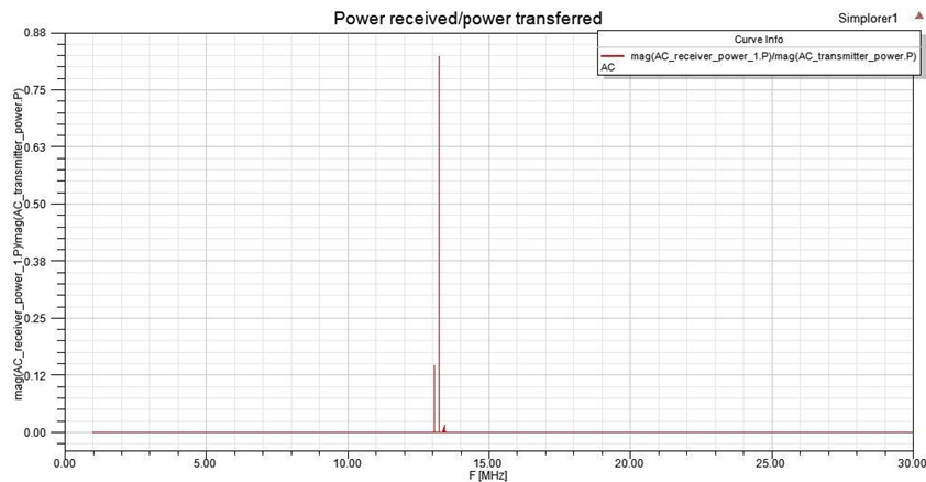
Figure 16: Ratio of power received per power transferred at resonance frequency
