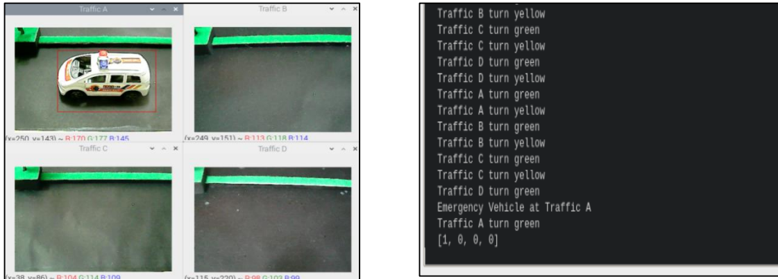
Figure 4: Left: ambulance detected in video streaming of webcam a, right: ambulance detected at traffic an updated by thonny shell
