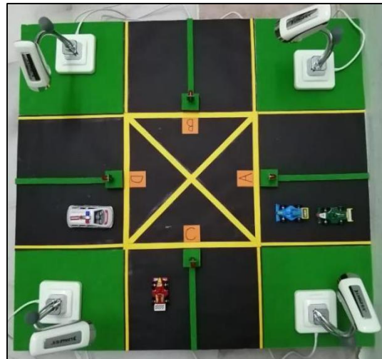
Figure 2: Prototype of 4 way traffic junction
