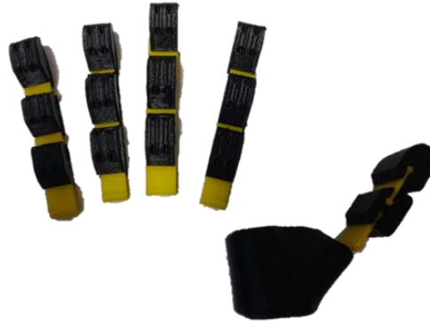
Figure 2: Fabrication of soft robot fingers
