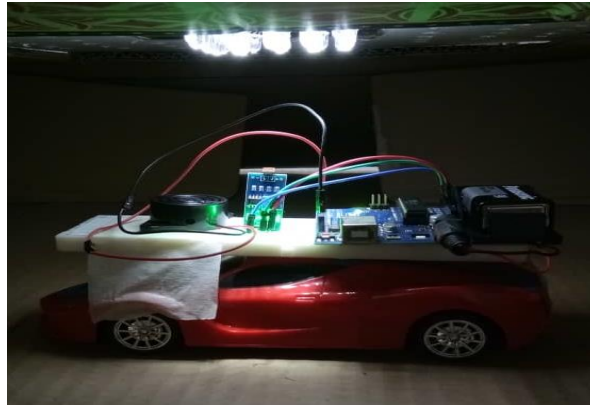
Figure 5: Prototype when LDR sensor was exposed to visible light
