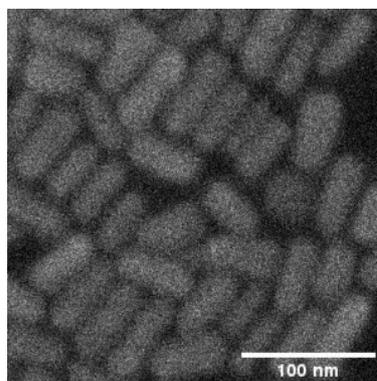
Figure 9: The FESEM image for GNRS with 0.1M CTAB
