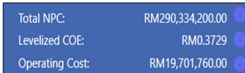
Figure 5: NPC, COE and operating cost of the grid-connected PV system and grid system
