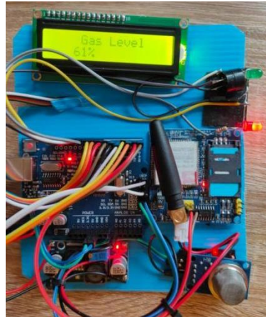
Figure 5: Device when the MQ-2 sensor detects the presence of gas leakage
