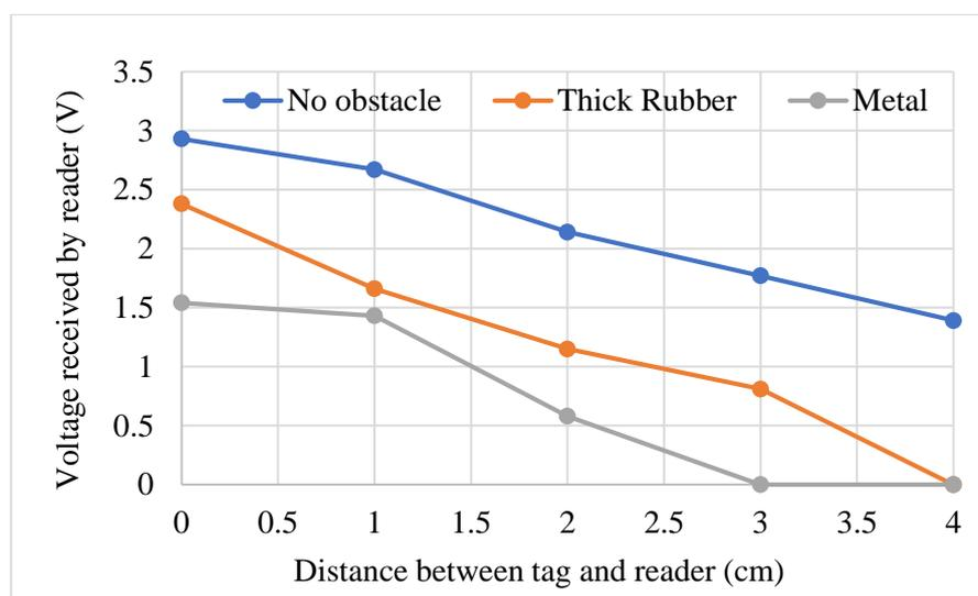
Figure 3: Graph of voltage received by reader vs distance (vertical)
