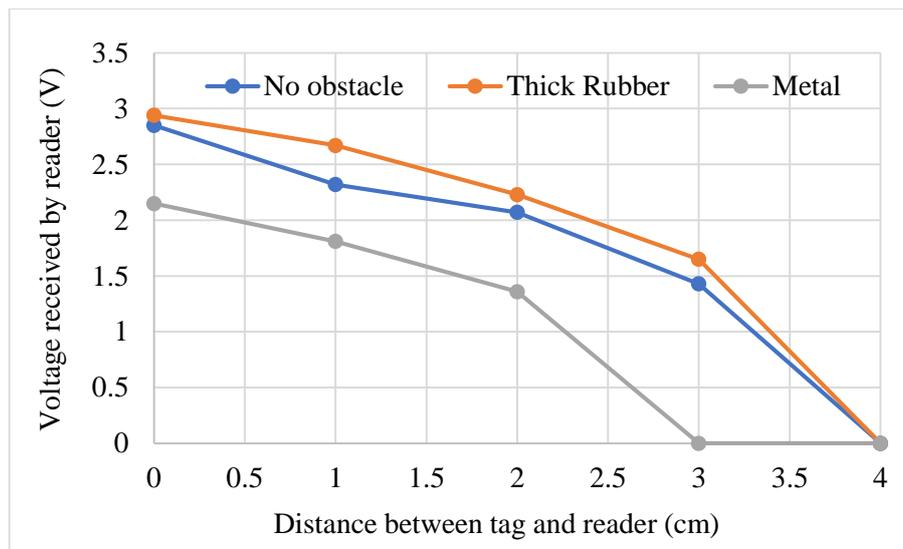
Figure 2: Graph of voltage received by reader vs distance (horizontal)
