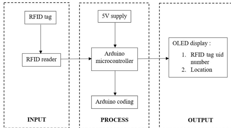
**Figure 1: Block diagram of RFID tagging system**
