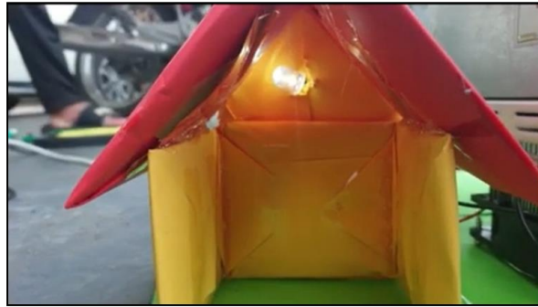
Figure 9: Lighting system supplied by the DC power system of the prototype
