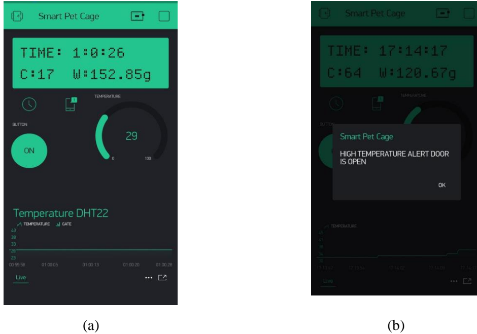
Figure 10: (a) Blynk profile of this project, (b) Notification that gate of the pet cage is open due to high temperature
