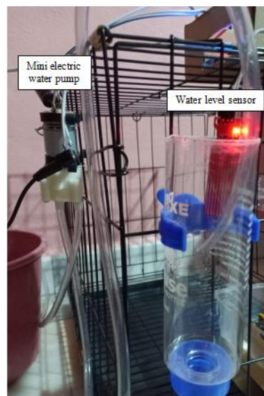
Figure 9: Arrangement of water level sensor and mini electric water pump
