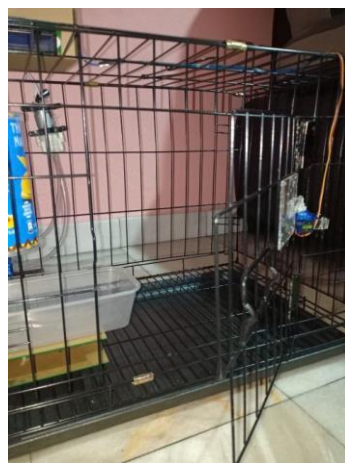
Figure 7: Gate of the cage open due to high temperature
