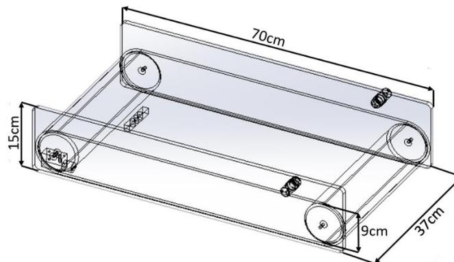
**Figure 2: Detail of conveyor belt design**
