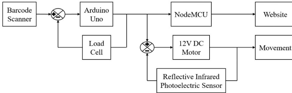
**Figure 3: Block diagram for electronic design**
