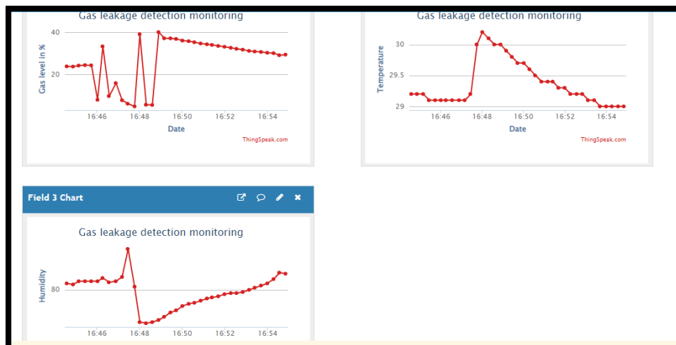
Figure 10: ThingSpeak data collection from gas leak detector
