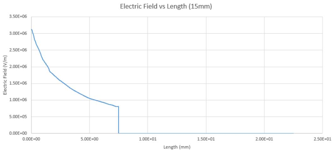
**Figure 13: The graph of electric field with 15mm arsenic powder**
