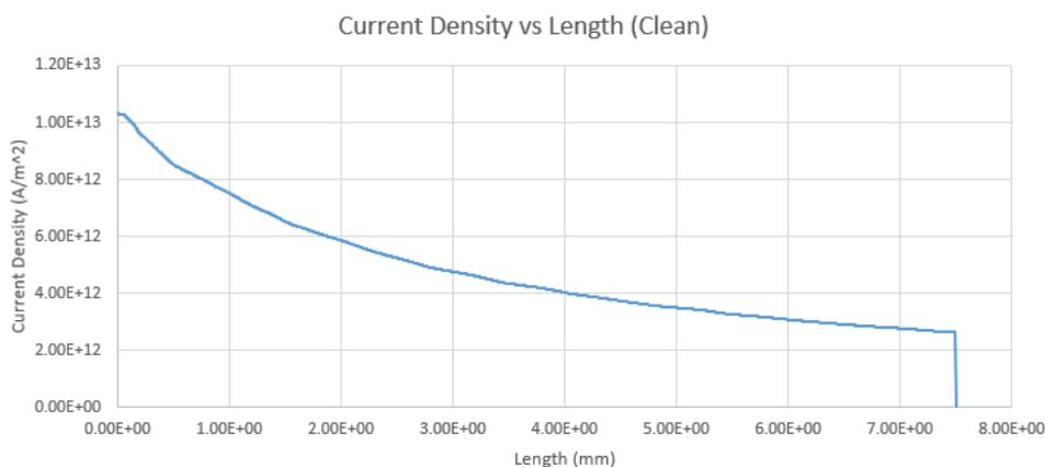
**Figure 8: The graph of current density of clean XLPE insulator cable**
