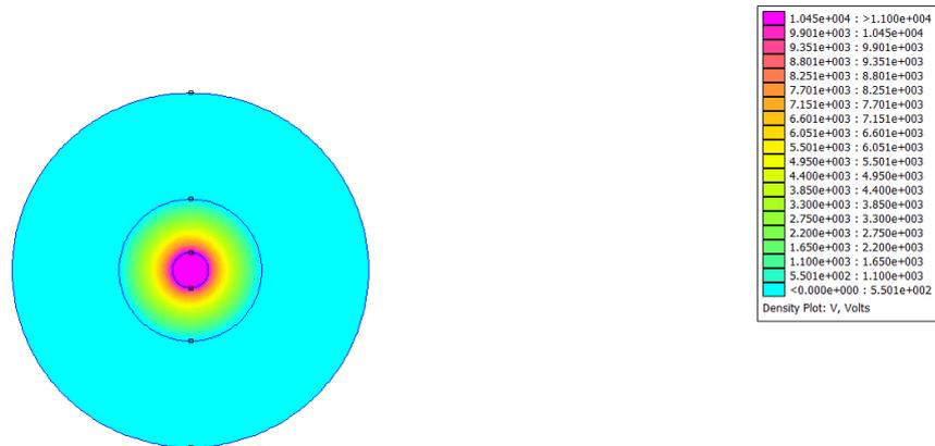
**Figure 6: The contoured cable image of insulator cable model with 15mm arsenic powder**
