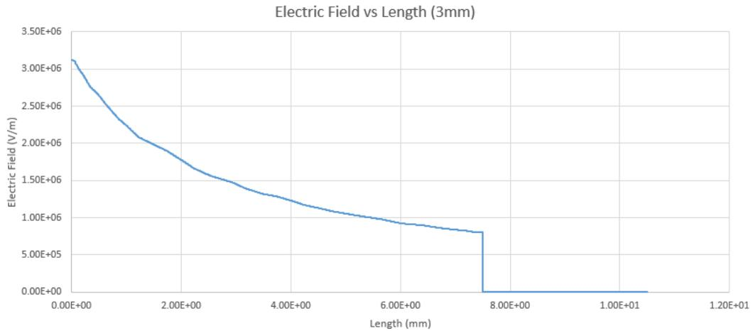
**Figure 9: The graph of electric field with 3mm arsenic powder**
