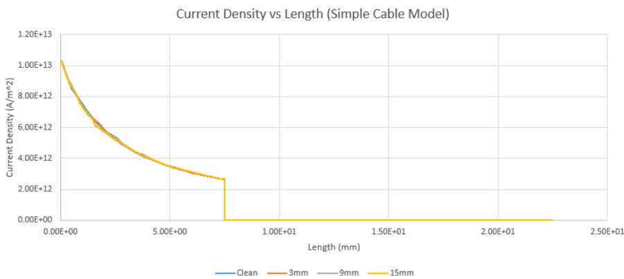
**Figure 16: The combination graph of current density for all thickness of arsenic powder**
