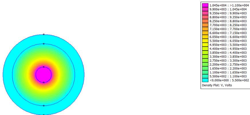
**Figure 4: The contoured cable image of the insulator cable with 3mm arsenic powder**
