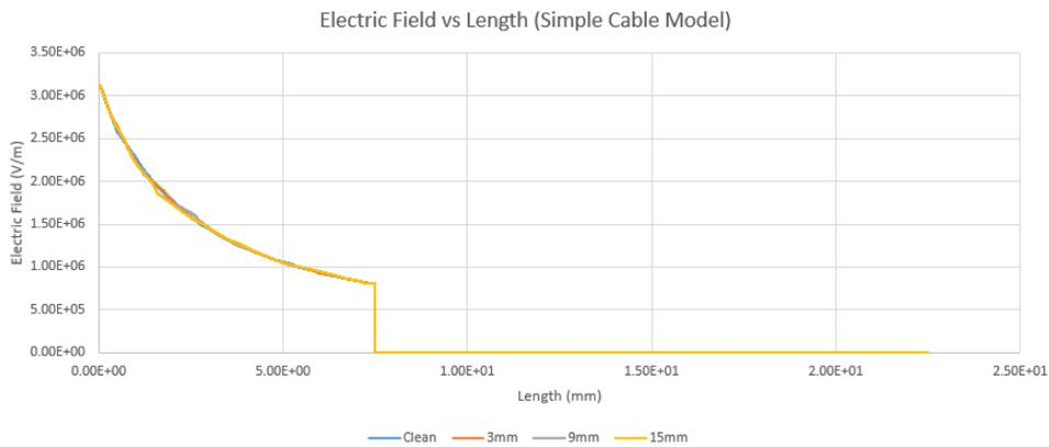
**Figure 15: The combination graph of electric field for all thickness of arsenic powder**
