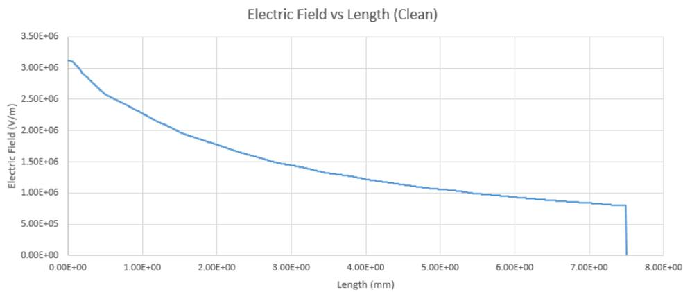
**Figure 7: The graph of electric field of clean XLPE insulator cable**
