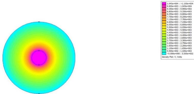
**Figure 3: The contoured image of insulator cable with no arsenic powder**
