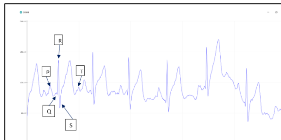
Figure 7: The ECG signal display at the serial monitor
