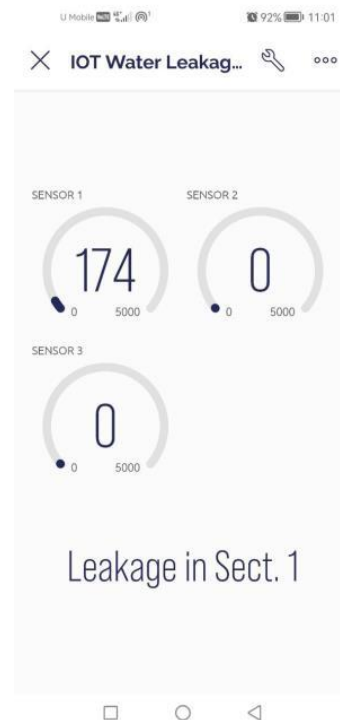
Figure 11: Blynk notification for leakage in section 1
