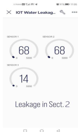
Figure 14: Blynk notification for leakage in section 2
