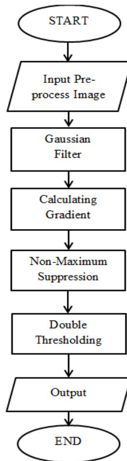
**Figure 3: Image segmentation flowchart**
