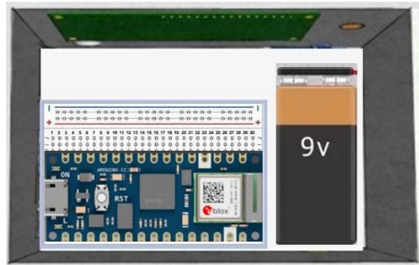
Figure 11: Packaging setup for Arduino nano BLE sense
