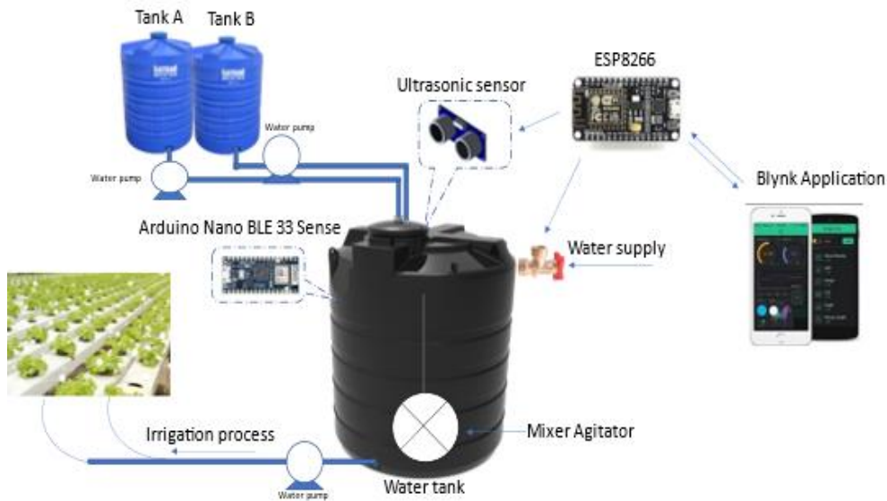
Figure 5: The layout of the automatic fertilizer system
