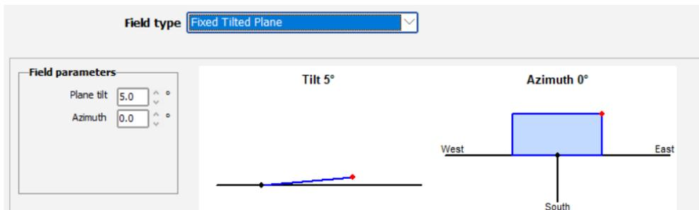
**Figure 2: Fixed tilt solar panel**
