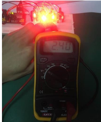
Figure 5: Red LED voltage reading
