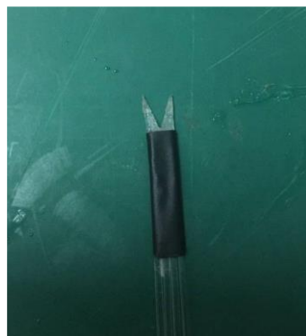
Figure 4: The design of POF surface 45 degree
