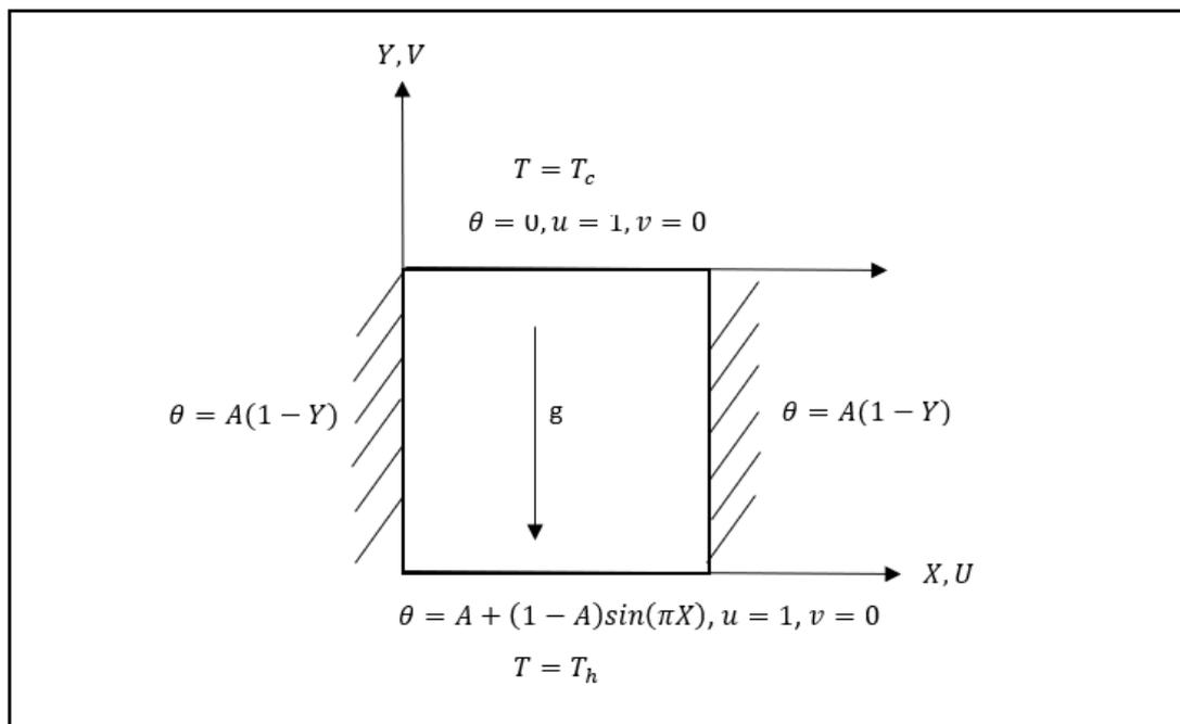
Figure 1: Schematic of the physical model for mixed convection within square cavity [5]
