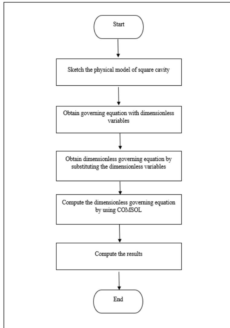
**Figure 2: Flow chart in using COMSOL Multiphysics 5.5**
