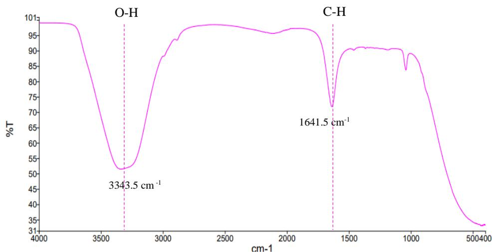
**Figure 3: FTIR spectrum of 3% of EPS embedded Cu nanoparticles**
