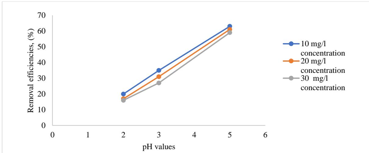
Figure 5: The effect of pH values of Zn heavy metals
