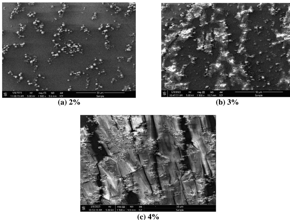
**Figure 1: FESEM micrographs of a) 2%, b) 3% and c) 4% of EPS embedded with  $\text{CuSO}_4 \cdot 5\text{H}_2\text{O}$**
