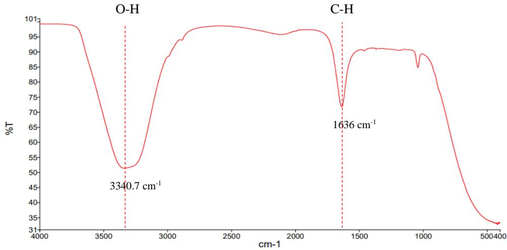
Figure 4: FTIR spectrum of 4% of EPS embedded Cu nanoparticles
