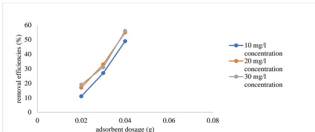
**Figure 6: The effect of different adsorbent dosages on Zn heavy metals**
