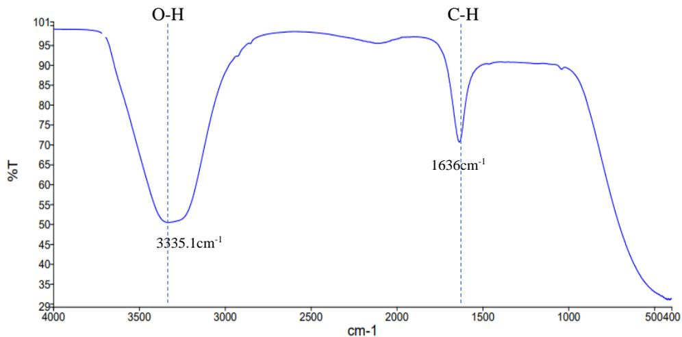
**Figure 2: FTIR spectrum of 2% of EPS embedded Cu nanoparticles**
