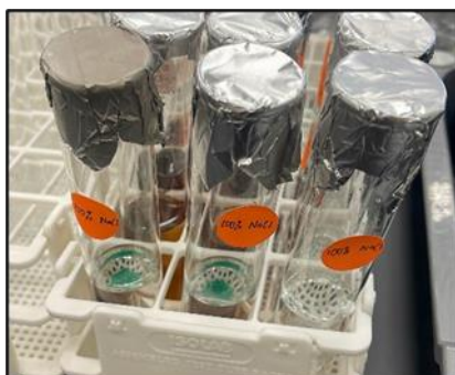
Fig. 4 Immersion of PCB in NaCl solutions with varying concentrations of PLE
