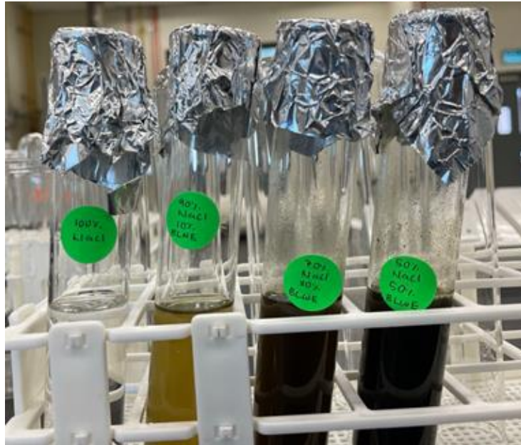
Fig. 4 Immersion of X70 steel samples inside of the different percentages NaCl solution and BLWE inhibitor in the test tubes
