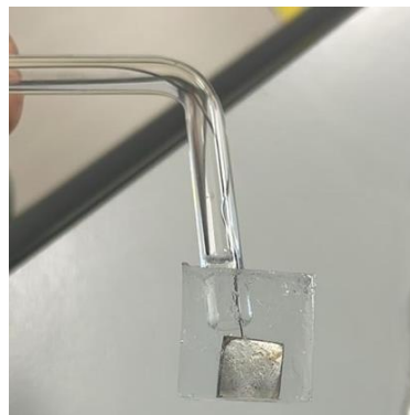
Fig. 5 X70 steel samples after the epoxy mounting and drying process
