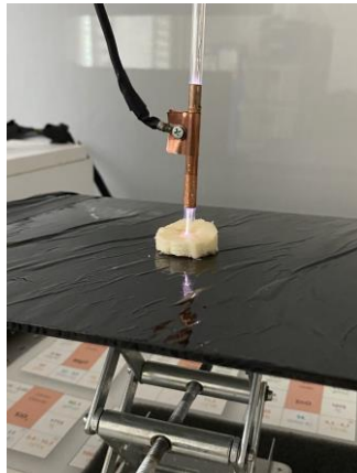
Fig. 2 setup of cold atmospheric plasma jet
