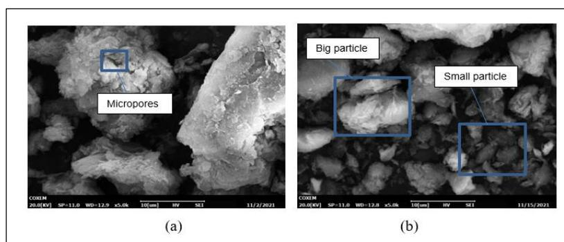
**Figure 7: (a) The morphology structure of Kulai-Yong Peng from SEM analysis, (b) The morphology structure of Rengam- Jerangau from SEM analysis**
