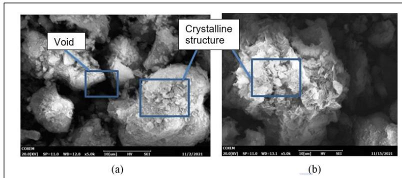
Figure 6: (a) The morphology structure of peat from SEM analysis, (b) The morphology structure of Selangor-kangkong from SEM analysis
