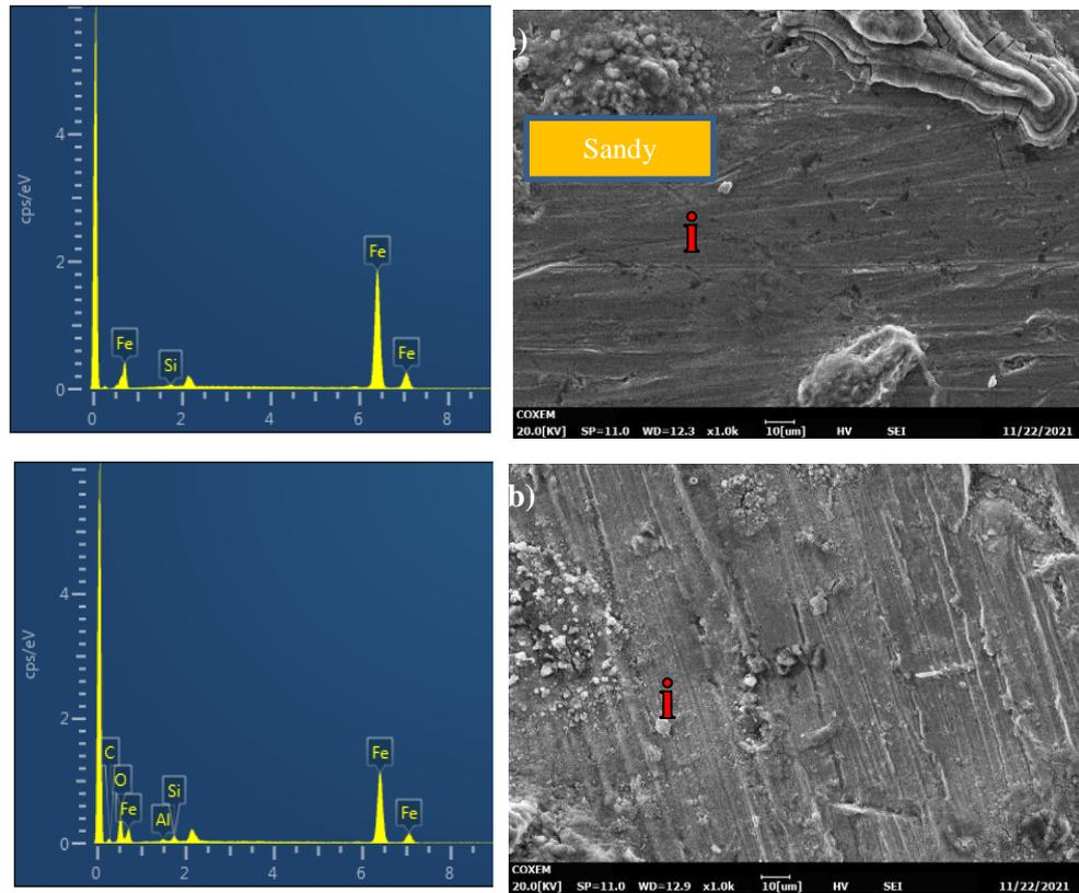
**Figure 5: SEM micrographs obtained on APL X70 pipeline steel in sedentary soil a) for 7 days and b) for 14 days**
