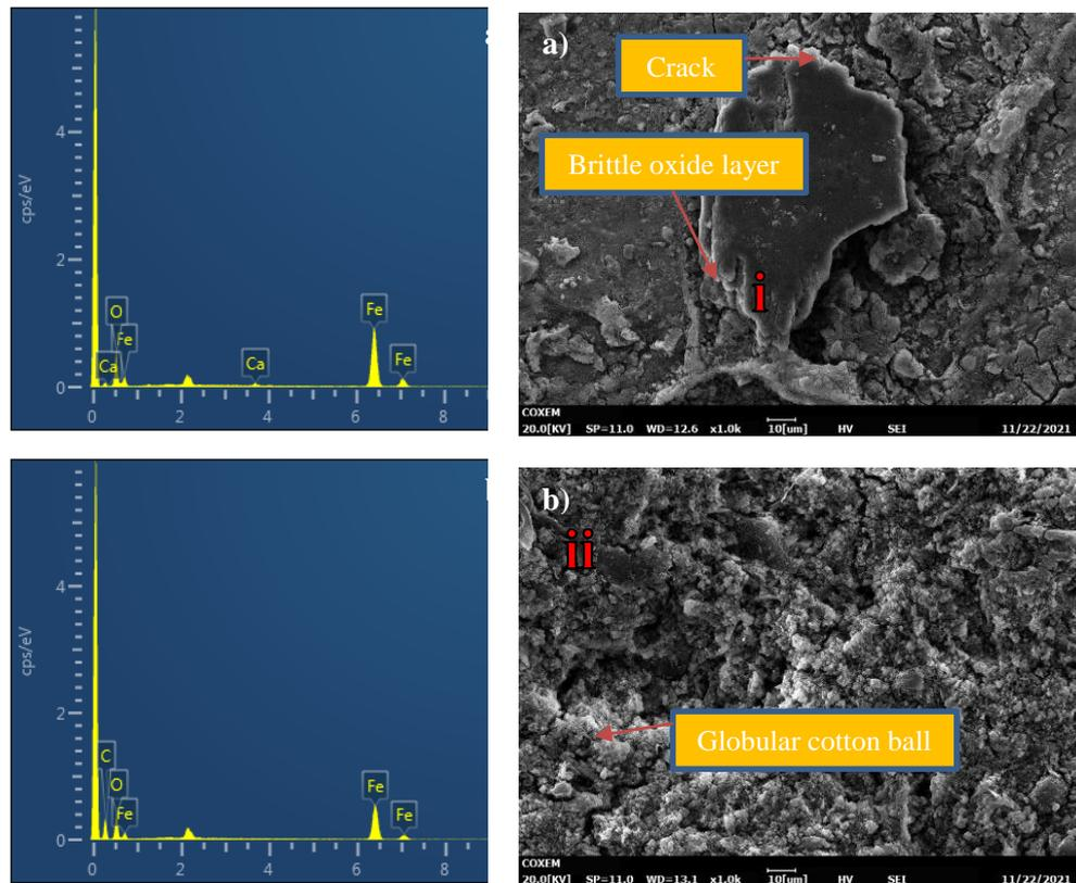
Figure 4: SEM micrographs obtained on APL X70 steel pipeline in peat soil a) for 7 days and b) for 14 days
