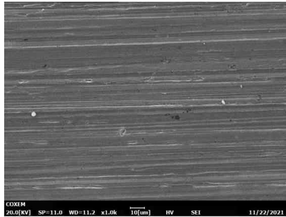
**Fig. 2: Polished of X70 steel pipeline**
