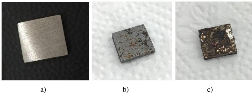
**Figure 1: Appearance of pre and postexposure samples; a) polished, b) exposed under sedentary, and c) exposed under peat soil**
