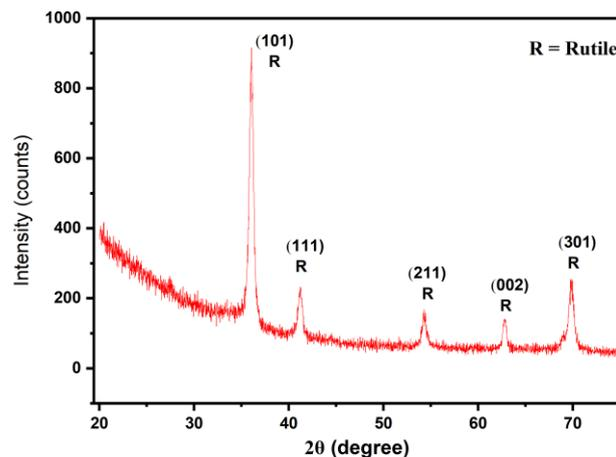
**Figure 1:** XRD patterns result of TiO<sub>2</sub> nanorods for reaction temperature of 150°C
