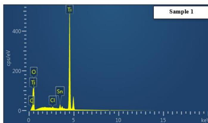
**Figure 2: The EDX analysis graph of TiO<sub>2</sub> nanorods for a reaction temperature of 150°C**
