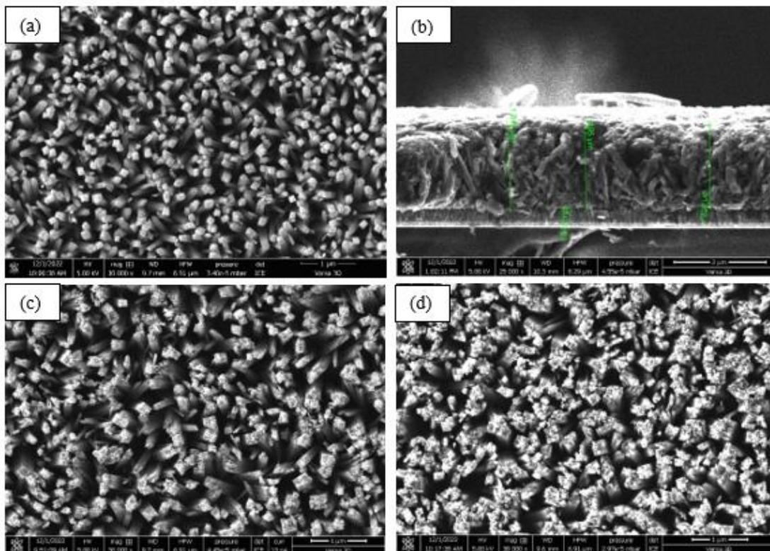
**Figure 3: FESEM results of TiO<sub>2</sub> nanorods surface morphology for (a) 150 °C (c) 170 °C and (d) 180 °C while (b) cross-sectional image for 150 °C**
