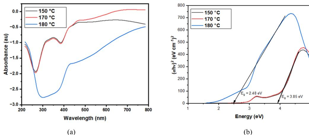
**Figure 6: (a) UV – Vis absorbance spectra of TiO<sub>2</sub> nanorods and (b) optical band gap of TiO<sub>2</sub> nanorods with different reaction temperatures from 150 °C, 170 °C and 180 °C**
