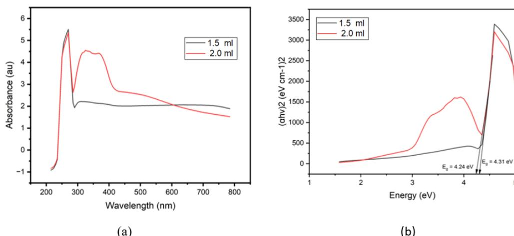
**Figure 8: (a) UV – Vis absorbance spectra of TiO<sub>2</sub> nanorods and (b) optical band gap of TiO<sub>2</sub> nanorods with different concentrations of TBOT from 1.5 ml and 2.0 ml**
