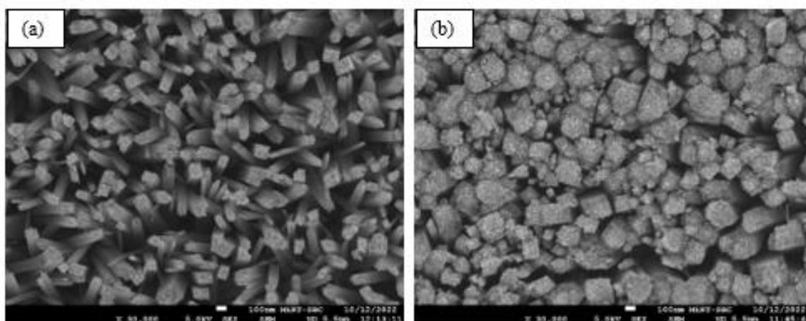
**Figure 5: FESEM results of TiO<sub>2</sub> nanorods surface morphology for (a) 1.5 ml concentration of TBOT and (b) 2.0 ml concentration of TBOT**
