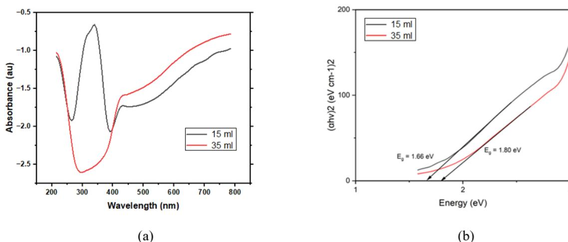
**Figure 7: (a) UV – Vis absorbance spectra of TiO<sub>2</sub> nanorods and (b) optical band gap of TiO<sub>2</sub> nanorod with different concentrations of HCl from 15 ml and 35 ml**
