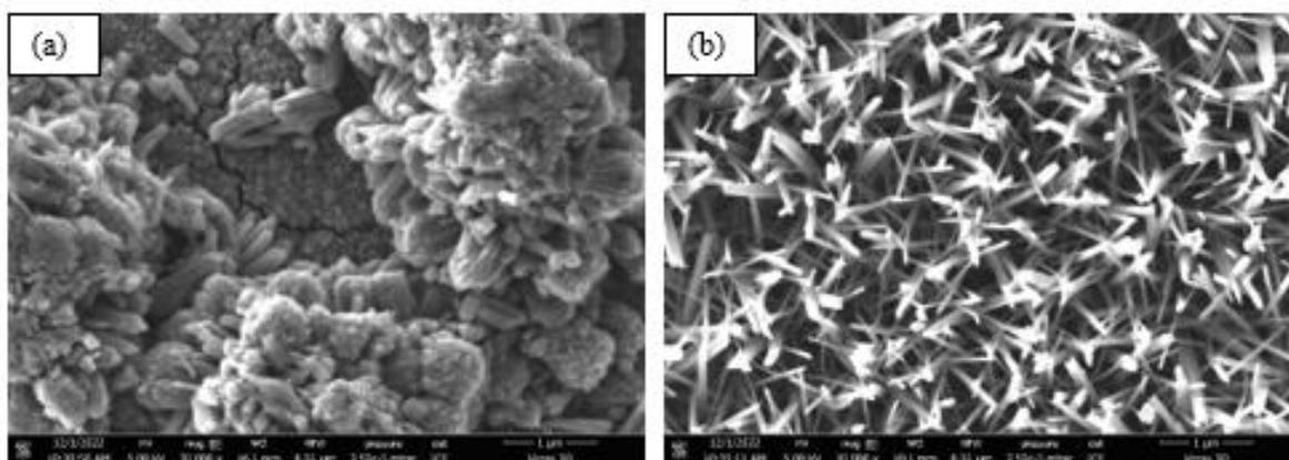
**Figure 4: FESEM results of TiO<sub>2</sub> nanorods surface morphology for (a) 15 ml concentration of HCl and (b) 35 ml concentration of HCl**
